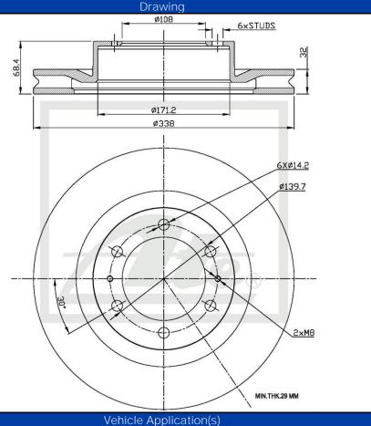
Brake Disc - FRONT Brake Disc Dimensions: Diameter - 338mm Height - 68.4mm
